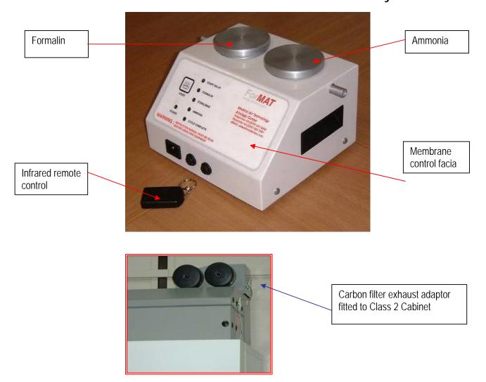
The For*MAT* Twin Fumigation Ammonia Neutralisation System is the solution to safety cabinet fumigation when, due to cabinet location, it is impossible to exhaust fumes to atmosphere.
